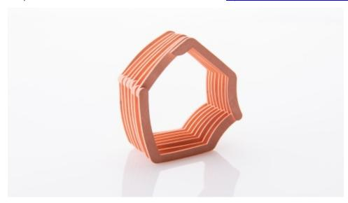
ExOne and Maxxwell Motors have successfully proved out a new concept for binder jet 3D printing a high-efficiency copper e-winding design that eliminates many of the challenges that come with traditional manufacturing of copper coils for electric motors. This new process eliminates the need for traditional coil wrapping, bending, tooling, and other inefficient process steps, also improving final part performance. (Graphic: Business Wire)
