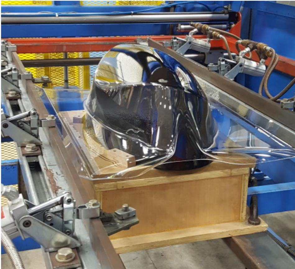
The ExOne Company now offers fast, durable, and affordable AMClad® Tooling. Developed by Ohio-based startup Freshmade 3D, AMClad is a patented process of infiltrating and coating 3D printed sand forms to give them strength for a wide range of tooling applications, including vacuum forming and more. (Photo: Business Wire)
