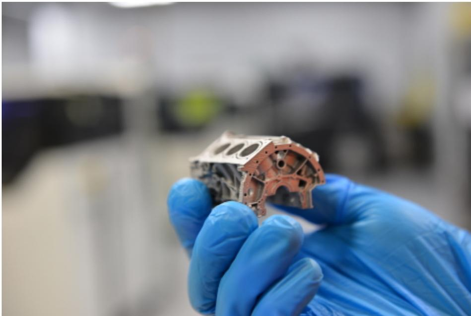
A new patent-pending process to binder jet 3D print and sinter the material delivers rapid and repeatable results: 99% density and material properties comparable to die casting. Additional collaborative and individual patents are expected to be filed by Ford and ExOne as a result of the ongoing project, as detailed in today's [simultaneous announcement](#).
