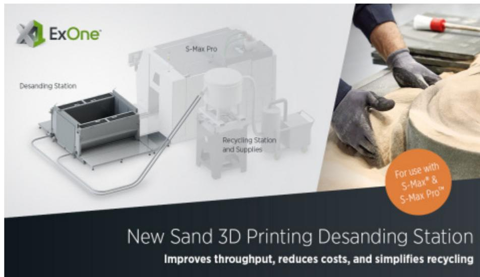
The new desanding station features two vacuum-powered wings that flank the job box and help easily remove excess sand as the build platform rises and parts are removed from the job box. The semi-automatic system is ideal for printers processing furan and CHP binders with fine or coarse grain silica sands or Cerabeads®, a premium ceramic foundry sand.
